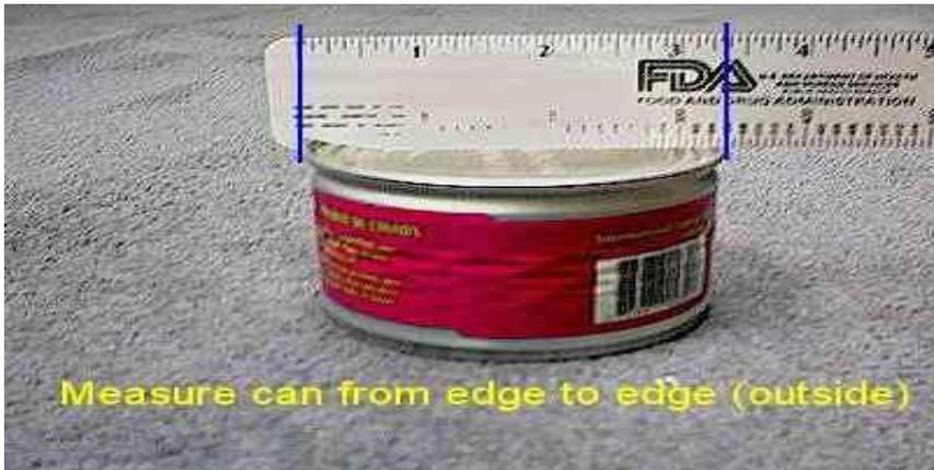
**Figure 41 – Measurement of Outer Edges of Container**
