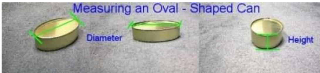
**Figure 40 – Measurement of an Oval Shape Container**
