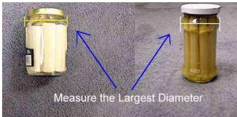
**Figure 39 – Measurement of an Unusual Shape Cylindrical Container.**
